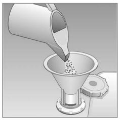
The LOW SALT indicator 5 on the front panel will light up initially but will extinguish again after a short period when the salt solution has become sufficiently concentrated
